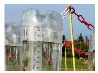
According to our flow model and our previous experiments, the flow rate expressed in % of the captive air in the bottle is very close to the evapotranspiration curve. The data was processed with a spreadsheet to plot the flow and water demand ET on a single graph. Here are the results of the test in Payerne between August 16 and August 20, 2018:
