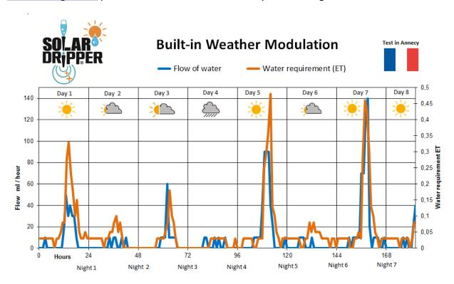
These ET evapotranspiration values are calculated from the weather measurements by the Penman-Monteith formula from a FAO standardized equation.
