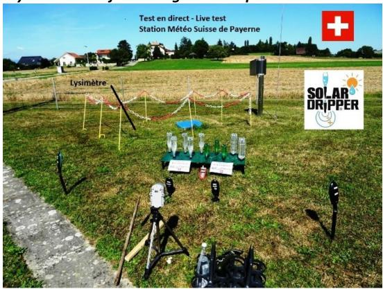
Tests were first carried out in Canada and in France to verify the synchronism of the Solar-Dripper flow with the needs of the plant. It <u>seemed very good</u> and the <u>plant growth was excellent</u>. Our first precise water requirement values came from ETp evapotranspiration calculations made from a <u>Davis Vantage Pro 2</u> professional weather station and by a WatchDog ET weather station.
