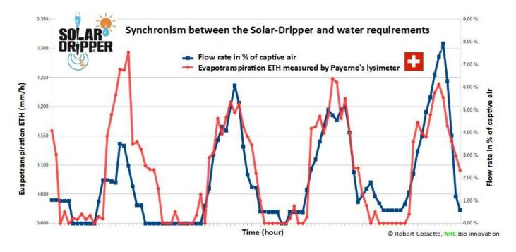
**Conclusion:** the correlation curves obtained demonstrate a natural tendency of the Solar-Dripper to follow the watering needs of the plant. Between a Solar-Dripper (costs less than 10 €) and a top class scientific lysimeter the curves are very close.
